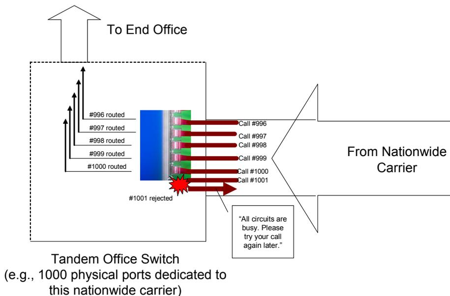
Figure 2 - Limited Physical Ports in Tandem Switch
