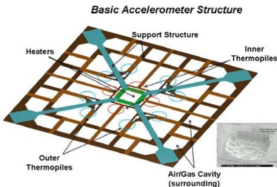
With no moving parts, MEMSIC’s accelerometers are longer-lasting, more reliable, and as much as 25 times more shock-resistant (up to 100,000 g) than their mechanical counterparts for measuring tilt, inclination, shock, and vibration. The chips appear in products that require the control or measurement of motion, such as car alarms, mobile electronics, global positioning systems, elevator
